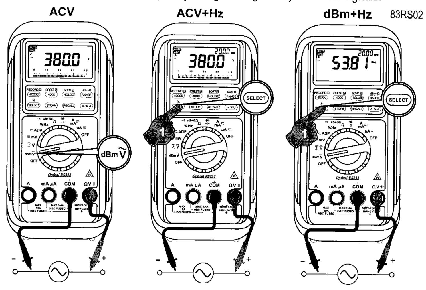
Note: Default Reference impedance  $600\Omega$  will be displayed for 2 seconds before displaying the dBm + Hz readings. Press **dBm-** $\Omega$  (**RANGE**) button momentary to select different reference impedance from 4, 8, 16, 32, 50, 75, 93, 110, 125, 135, 150, 200, 250, 300, 500, 600, 800, 900, 1000, up to  $1200\Omega$ . Impedance values will again be displayed for 2 seconds before displaying the dBm + Hz readings.
