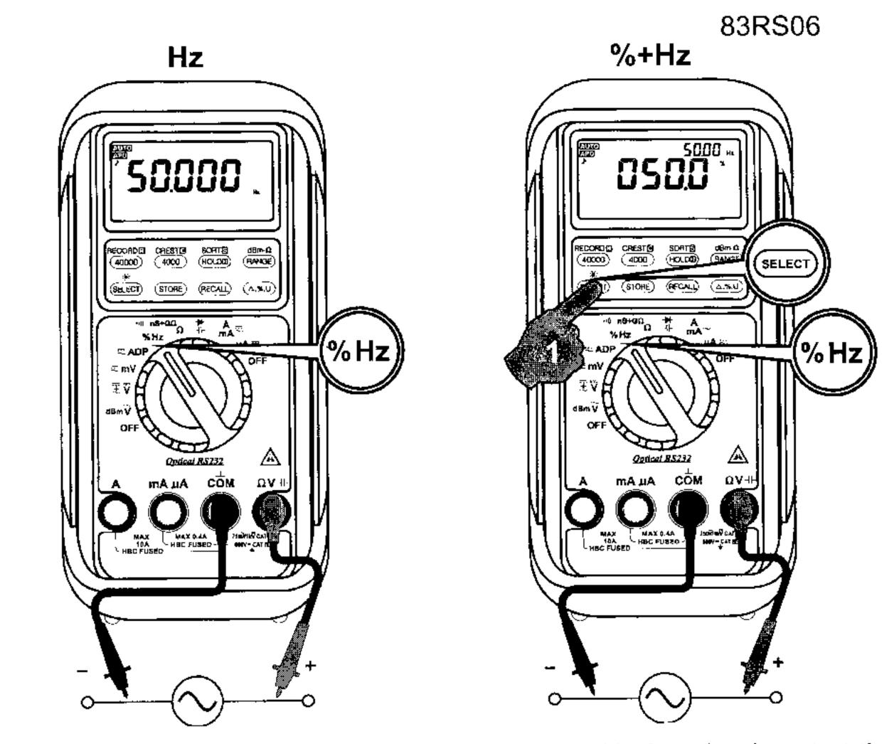
Note: Unlike the AC + Hz function, this high resolution Hz function is set at the highest input sensitivity to measure digital type electronic signals.
